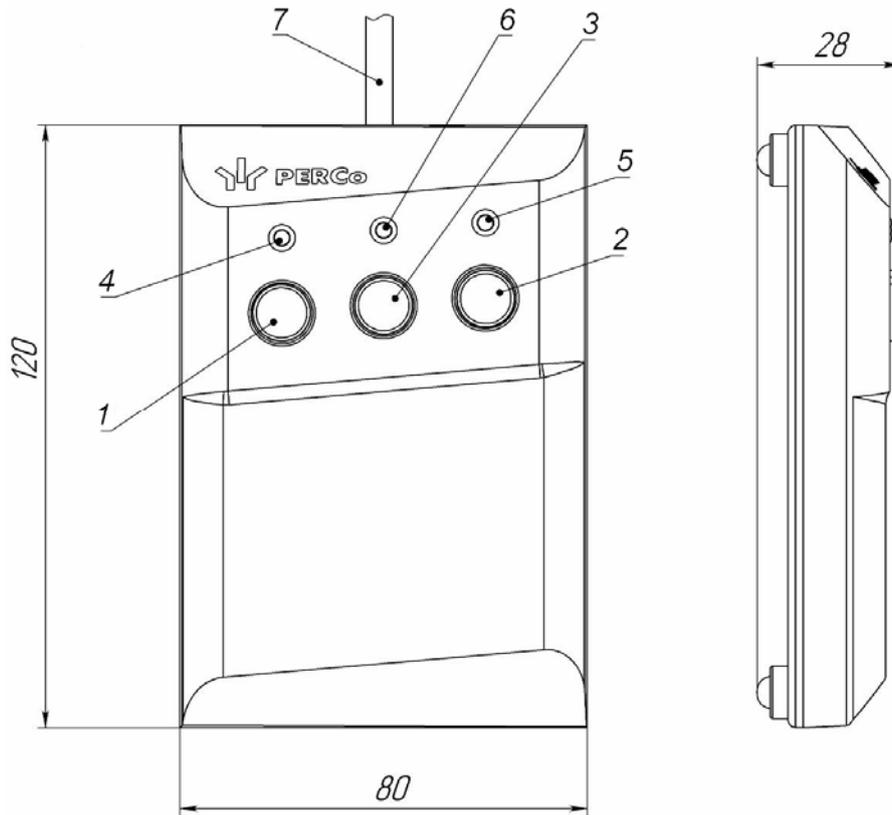
**Figure 3. RC panel overall view**
