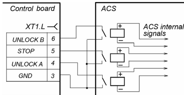
**Figure 5. ACS control element — normally open relay contact**
