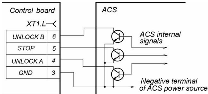
**Figure 6. ACS control element — circuit with open-collector output**
