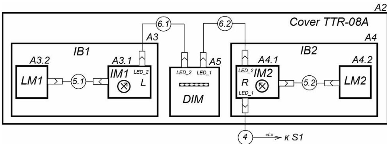
Figure 13. Turnstile cover connection layout
